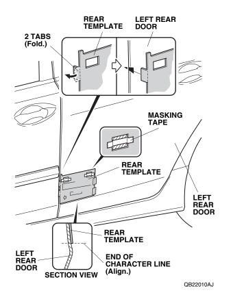
12. Align the rear template with the end of the character line, and attach it to the left rear door using strips of masking tape.
