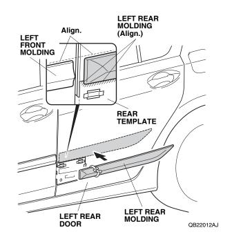
15. While applying light pressure against the left rear molding, carefully remove the two adhesive backings.
