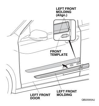
6. While applying light pressure against the left front molding, carefully remove the two adhesive backings.
