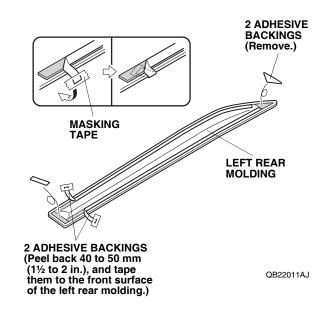
14. Align the left rear molding with the rear template and the left front molding, and attach it to the left rear door.
