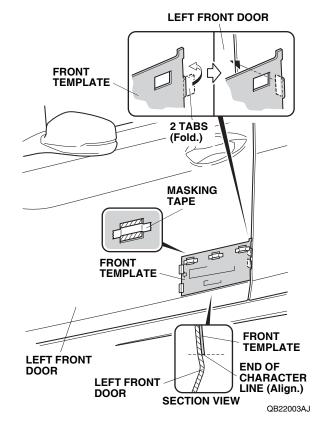
3. Align the front template with the end of the character line, and attach it to the left front door with strips of masking tape.
